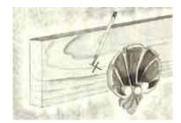
Drill pilot holes through the surface of the work at the marked points.
