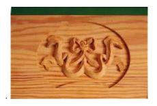
Craftsman's tip - Route out a rebate to approximately the same depth as the carving to be highlighted, plus a couple of centimetres wider in diameter. Fix the carving to lie flat inside the rebate, gluing it in place. It will appear to have been carved directly into the surrounding wood.
